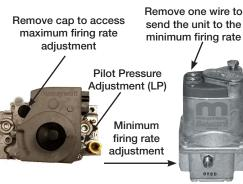
Fig. 2 Separate Regulator and Modulating Valves
