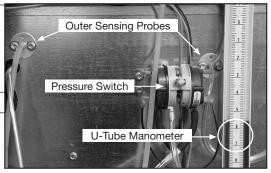
Fig. 1 Measuring the Pressure Drop
